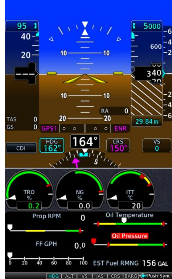
Figure 7-2: Single Engine Turboprop Display Backup
