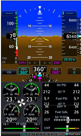
Figure 7-1: Twin Piston Display Backup
