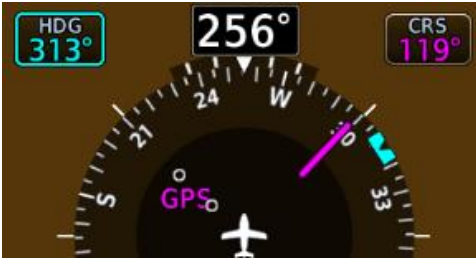
Figure 4-2: Magnetic Navigation Angle (System Default)
