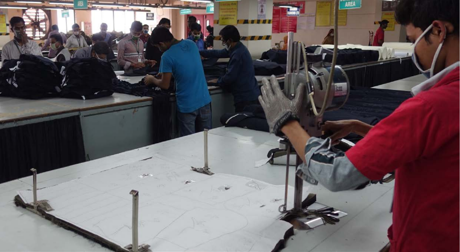
Picture 3. Cutting of details of a garment, a small side-lay in regular production in a factory in Bangladesh
